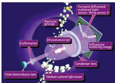
Optical system in SALD-7500nano
